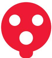
**Commando:** these are often used on commercial or industrial sites where more power is required than a normal UK 3-pin plug.
