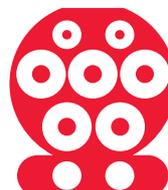
**CCS (Combo 2):** Widely used in Europe, this is a version of type 2 connector with two additional power contacts. It allows very fast charging. This socket is always combined with either a Type 2 or a Type 1 socket.
