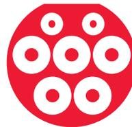
**Type 2:** this is the standard for European and Asian vehicles (Nissan Leaf for example) from 2018 onwards. It's by far the most common and can charge at a level of up to 43 kW.
